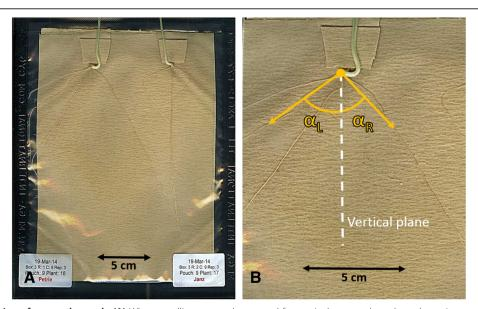
**Figure 7 Illustration of a growth pouch. (A)** Wheat seedlings were phenotyped for seminal root angle and number using growth pouches (picture taken 20 days after sowing). **(B)** For each plant, the left  $(\alpha_L)$  and the right  $(\alpha_R)$  angle between each of the first pair of seminal roots and the vertical plane was measured at approximately 3 cm distance from the seed using software (*Opengelphoto*).
