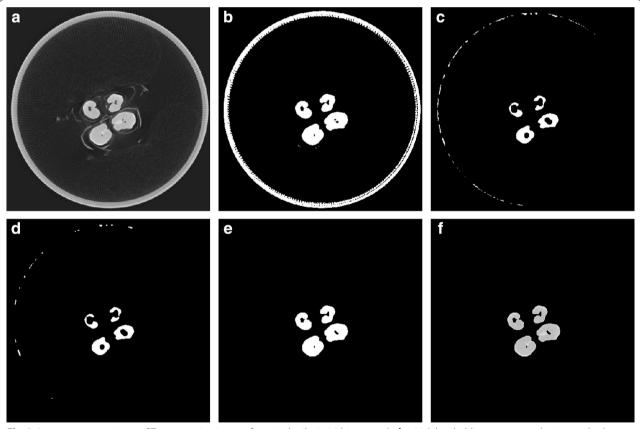
Fig. 3 Image segmentation. **a** µCT cross section image of a typical spike in 16-bit greyscale, **b** initial thresholding using our adaptive method, **c** erosion to remove outlying objects using a disk structuring element (SE), **d** median filter applied to smooth and further segment region of interest (ROI), **e** image dilated by same SE as (**c**) and with remaining holder removed and **f** final result of this process was obtained by using (**e**) as a mask in conjunction with (**a**)
